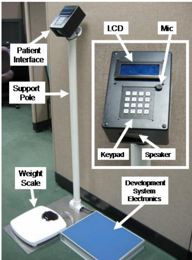
Figure 4. Assembled Patient Scale development system with pole mounted patient interface. Insert shows detail of patient interface unit.
