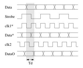
**Fig. 5**. Receiver waveform for mesochronous transmission.  $T_d$  denotes the receiver synchronization delay.
