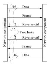
**Fig. 2**. Basic signals for one undirectional internal network link.
