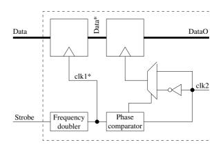
Fig. 4. Receiver for strobed mesochronous clocking.
