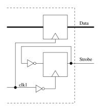
Fig. 3. Sender for strobed mesochronous clocking.
