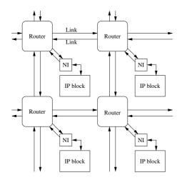
Fig. 1. Section of a mesh style on-chip network.
