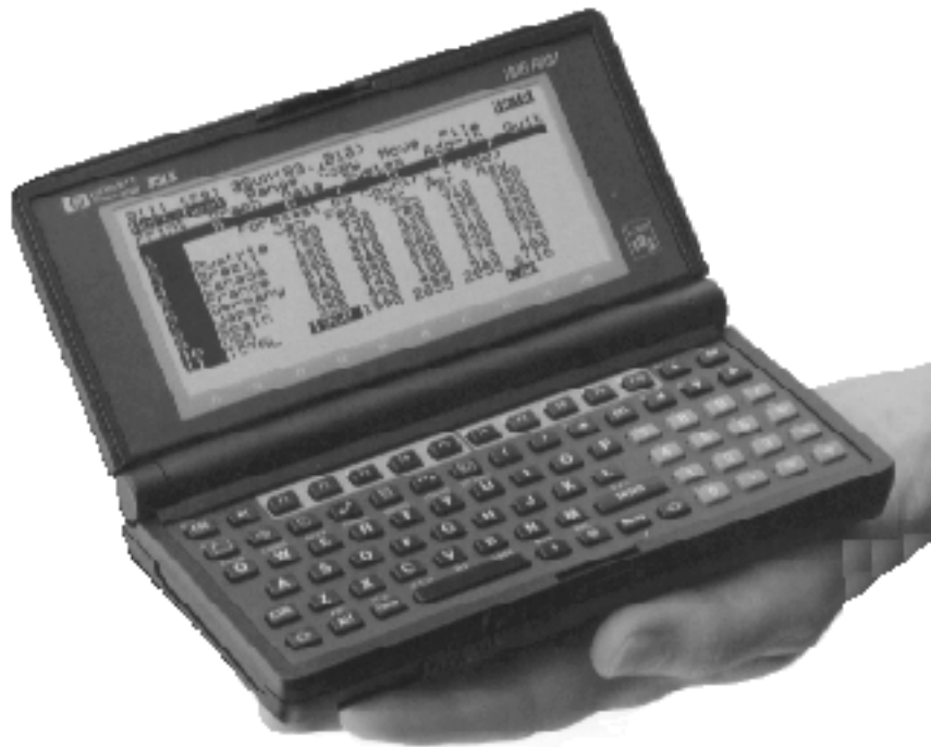
Figure 1. The HP 95LX is small enough to fit in the user's palm. The machine comes with 1MB of RAM, runs MS-DOS, and has a 2400 baud IR I/O port.
