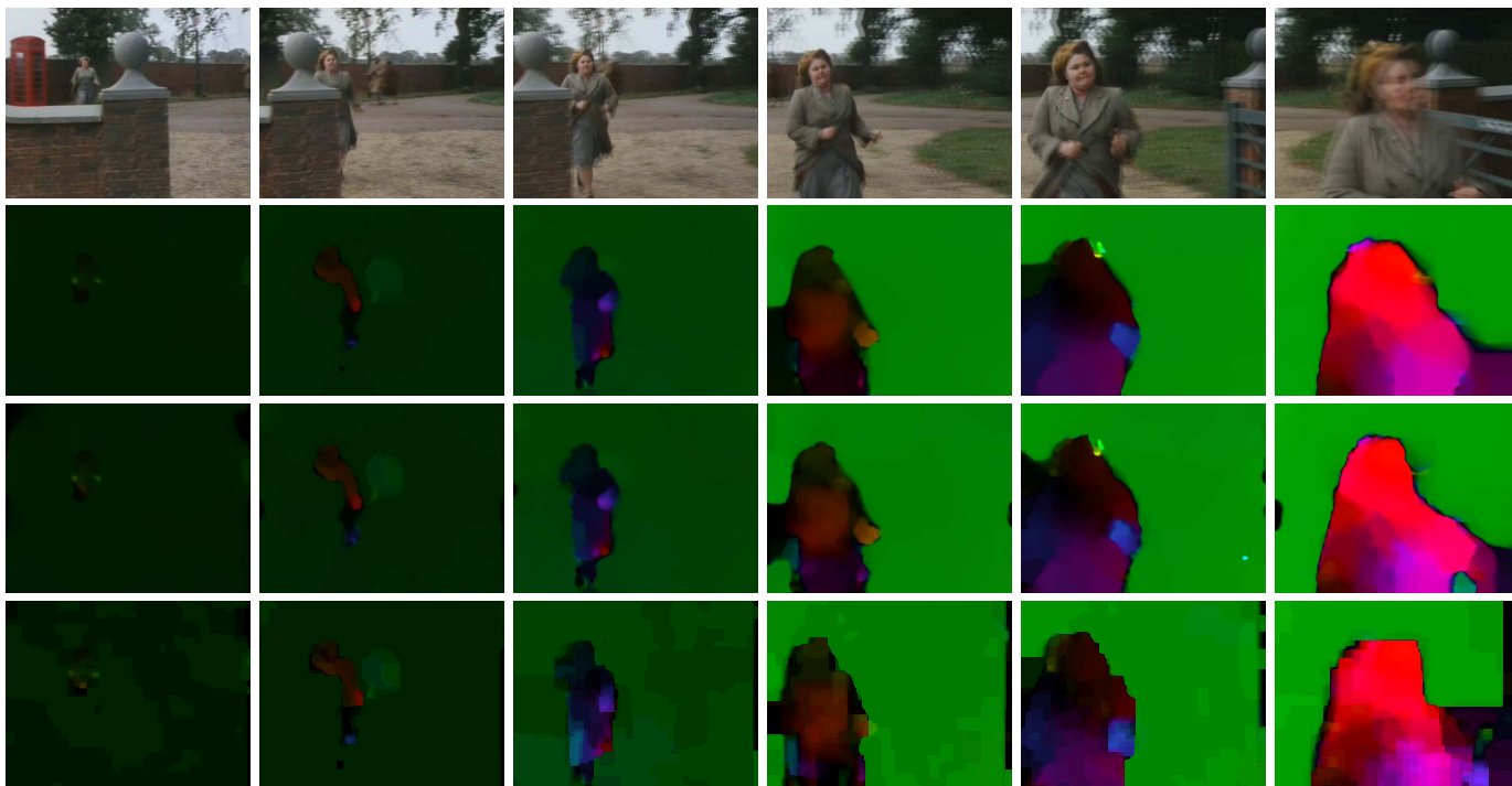
Fig. 8. Shot from Miss Marple: A pocket full of rye . First row: Input pairs overlaid to visualize the motion. Second row: Classic warping [11]. Third row: Large displacement optical flow (LDOF). Fourth Row: SIFT flow [23]. The hand in the last frame actually moves to the left, which is only captured by LDOF.
