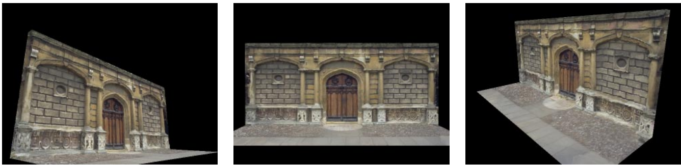
Figure 16: Novel views of the scene generated from four original photographs. These are frames from an animated movie in which the façade rotates continuously. The depth is computed from model-based stereo and the frames are made by compositing image-based renderings with view-dependent texture-mapping.
