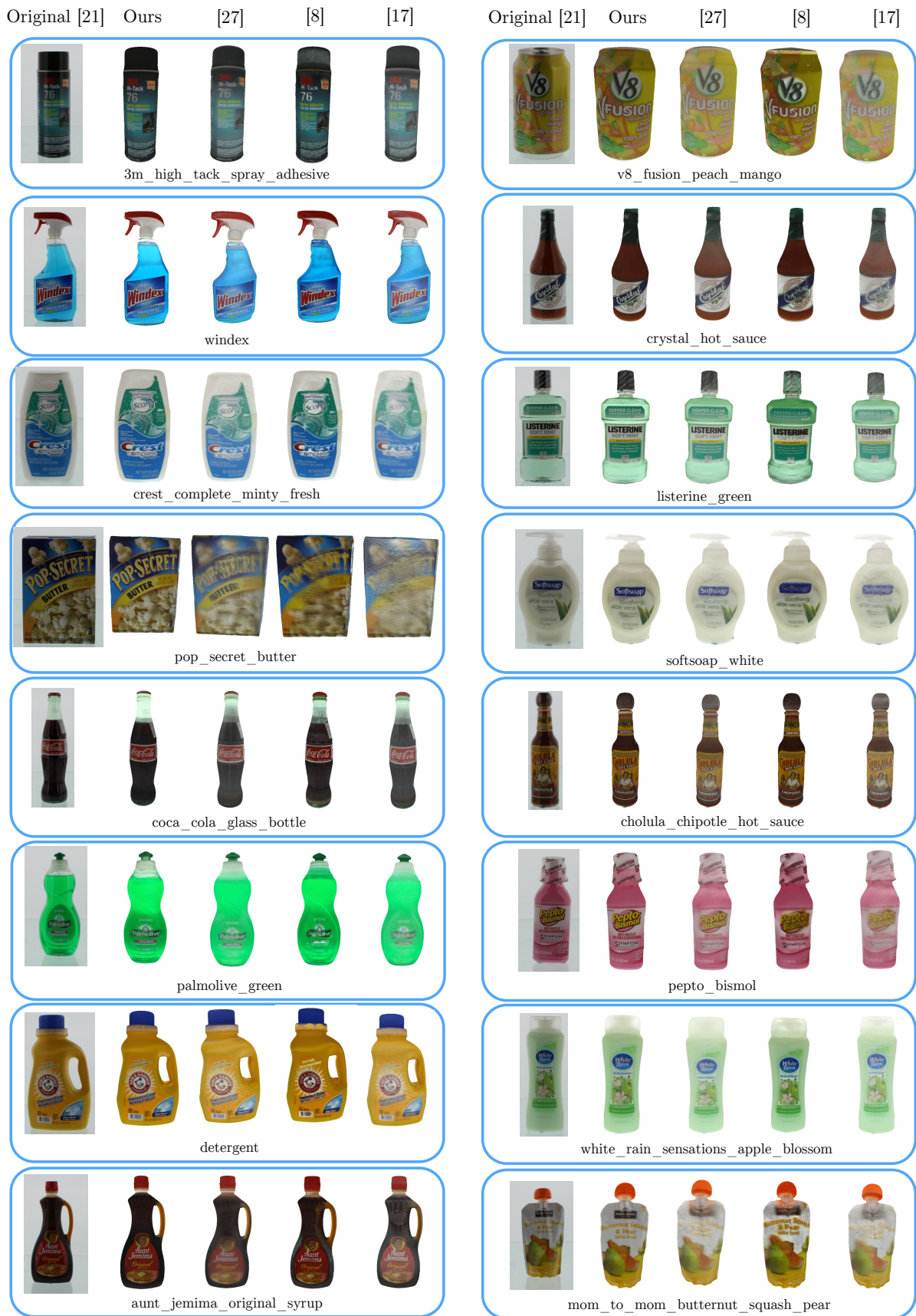
Fig. 7. Juxtapositions of original BigBIRD images [21] with color model reconstructions from (1) our method, (2) Zhou et. al. [27] without deformation grid optimization, (3) Hernandez et. al. [8], and (4) PCL's volumetric blending [17]. Note that we do not employ Zhou et. al.'s deformation grid optimization, since this leads to divergence. Please use a PDF reader's digital zoom to view details.
