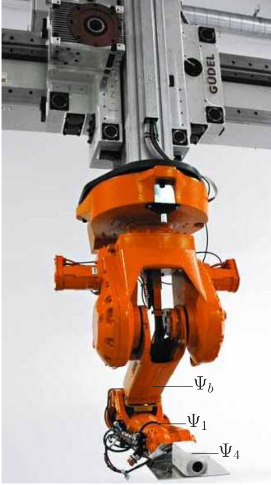
Fig. 5. ABB robot mounted on a gantry crane. The first 5 joints (the 3 of the gantry crane and the first 2 of the robot) are used to generate the ship motion and the last four joints of the robot are used for optimal motion planning of a 4-DoF robot. Links 2 and 3 of the robot are hidden in the wrist. Courtesy ABB Strategic R&D for Oil, Gas and Petrochemicals.
