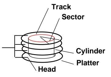
3600 RPM = 60 RPS => 16 ms per rev ave rot. latency = 8 ms 32 sectors per track => 0.5 ms per sector 1 KB per sector => 2 MB / s 32 KB per track 20 tracks per cyl => 640 KB per cyl 2000 cyl => 1.2 GB
