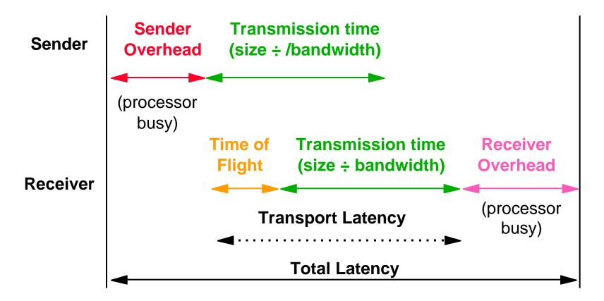
Total Latency = Sender Overhead + Time of Flight + Message Size ÷ BW + Receiver Overhead
