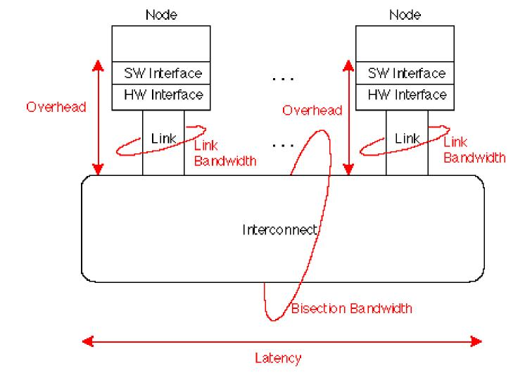
• Overhead: latency of interface vs. Latency: network 396 31
