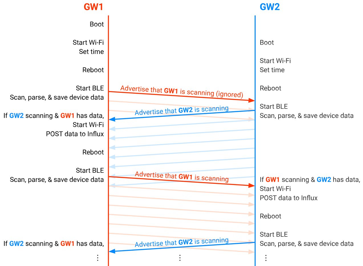
Figure 3.5: Timing diagram of the coordinated approach. Depicts communication between two gateways (GW1 & GW2).
