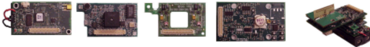
Fig. 8. Sensor hardware from left to right: (a) Mica2 network node, (b) Mica Sensor Board, (c) Mica Power Board, (d) TWR-ISM-002 Radar Board, and (e) All of the boards attached together.
