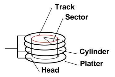
3600 RPM = 60 RPS => 16 ms per rev ave rot. latency = 8 ms 32 sectors per track => 0.5 ms per sector 1 KB per sector => 2 MB / s 32 KB per track 20 tracks per cyl => 640 KB per cyl 2000 cyl => 1.2 GB
