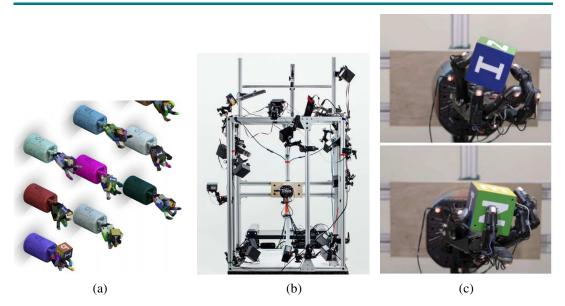
**Figure 26.26** Training a robust policy. (a) Multiple simulations are run of a robot hand manipulating objects, with different randomized parameters for physics and lighting. Courtesy of Wojciech Zaremba. (b) The real-world environment, with a single robot hand in the center of a cage, surrounded by cameras and range finders. (c) Simulation and real-world training yields multiple different policies for grasping objects; here a pinch grasp and a quadpod grasp. Courtesy of OpenAI. See ? (?).
