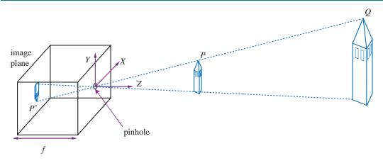
Figure 25.2 Each light sensitive element at the back of a pinhole camera receives light that passes through the pinhole from a small range of directions. If the pinhole is small enough, the result is a focused image behind the pinhole. The process of projection means that large, distant objects look the same as smaller, nearby objects—the point P' in the image plane could have come from a nearby toy tower at point P or from a distant real tower at point Q.
