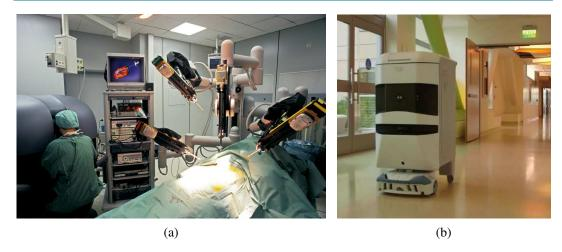
**Figure 26.34** (a) Surgical robot in the operating room. Photo by Patrick Landmann/Science Source. (b) Hospital delivery robot. Photo by Wired.
