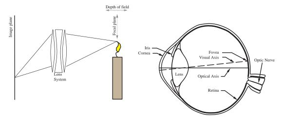
**Figure 25.3** Lenses collect the light leaving a point in the scene (here, the tip of the candle flame) in a range of directions, and steer all the light to arrive at a single point on the image plane. Points in the scene near the focal plane—within the depth of field—will be focused properly. In cameras, elements of the lens system move to change the focal plane, whereas in the eye, the shape of the lens is changed by specialized muscles.
