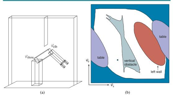
**Figure 26.12** (a) Workspace representation of a robot arm with two degrees of freedom. The workspace is a box with a flat obstacle hanging from the ceiling. (b) Configuration space of the same robot. Only white regions in the space are configurations that are free of collisions. The dot in this diagram corresponds to the configuration of the robot shown on the left.
