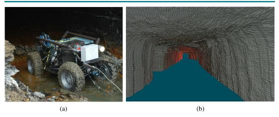
**Figure 26.36** (a) A robot mapping an abandoned coal mine. (b) A 3D map of the mine acquired by the robot. Courtesy of Sebastian Thrun.
