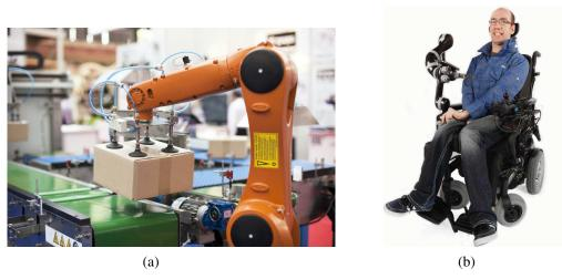
**Figure 26.1** (a) An industrial robotic arm with a custom end-effector. Image credit: Macor/123RF. (b) A Kinova<sup>®</sup> JACO<sup>®</sup> Assistive Robot arm mounted on a wheelchair. Kinova and JACO are trademarks of Kinova, Inc.
