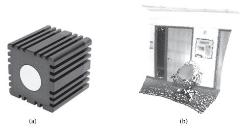
**Figure 26.3** (a) Time-of-flight camera; image courtesy of Mesa Imaging GmbH. (b) 3D range image obtained with this camera. The range image makes it possible to detect obstacles and objects in a robot's vicinity. Image courtesy of Willow Garage, LLC.
