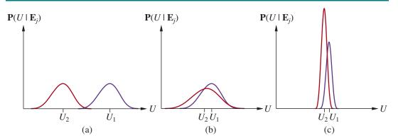
Figure 16.8 Three generic cases for the value of information. In (a),  $a_1$  will almost certainly remain superior to  $a_2$ , so the information is not needed. In (b), the choice is unclear and the information is crucial. In (c), the choice is unclear, but because it makes little difference, the information is less valuable. (Note: The fact that  $U_2$  has a high peak in (c) means that its expected value is known with higher certainty than  $U_1$ .)
