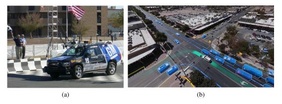
**Figure 26.35** (a) Autonomous car Boss which won the DARPA Urban Challenge. Photo by Tangi Quemener/AFP/Getty Images/Newscom. Courtesy of Sebastian Thrun. (b) Aerial view showing the perception and predictions of the Waymo autonomous car (white vehicle with green track). Other vehicles (blue boxes) and pedestrians (orange boxes) are shown with anticipated trajectories. Road/sidewalk boundaries are in yellow. Photo courtesy of Waymo.
