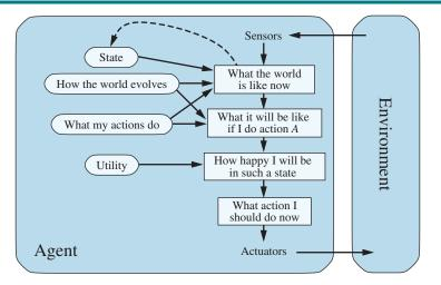
**Figure 2.14** A model-based, utility-based agent. It uses a model of the world, along with a utility function that measures its preferences among states of the world. Then it chooses the action that leads to the best expected utility, where expected utility is computed by averaging over all possible outcome states, weighted by the probability of the outcome.
