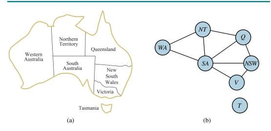
**Figure 6.1** (a) The principal states and territories of Australia. Coloring this map can be viewed as a constraint satisfaction problem (CSP). The goal is to assign colors to each region so that no neighboring regions have the same color. (b) The map-coloring problem represented as a constraint graph.
