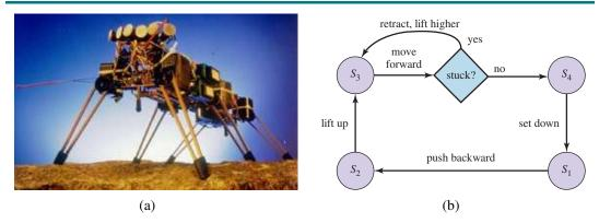
**Figure 26.32** (a) Genghis, a hexapod robot. (Image courtesy of Rodney A. Brooks.) (b) An augmented finite state machine (AFSM) that controls one leg. The AFSM reacts to sensor feedback: if a leg is stuck during the forward swinging phase, it will be lifted increasingly higher.
