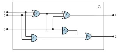
Figure 8.6 A digital circuit  $C_1$ , purporting to be a one-bit full adder. The first two inputs are the two bits to be added, and the third input is a carry bit. The first output is the sum, and the second output is a carry bit for the next adder. The circuit contains two XOR gates, two AND gates, and one OR gate.
