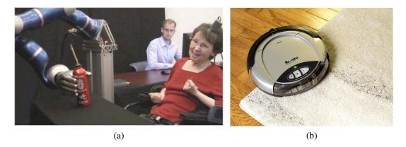
**Figure 26.33** (a) A patient with a brain–machine interface controlling a robot arm to grab a drink. Image courtesy of Brown University. (b) Roomba, the robot vacuum cleaner. Photo by HANDOUT/KRT/Newscom.
