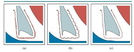
**Figure 26.22** Robot arm control using (a) proportional control with gain factor 1.0, (b) proportional control with gain factor 0.1, and (c) PD (proportional derivative) control with gain factors 0.3 for the proportional component and 0.8 for the differential component. In all cases the robot arm tries to follow the smooth line path, but in (a) and (b) deviates substantially from the path.
