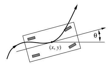
A car has more DOF (3) than controls (2), so is non-holonomic; cannot generally transition between two infinitesimally close configurations
