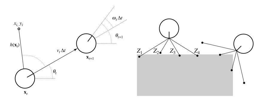
Assume Gaussian noise in motion prediction, sensor range measurements
