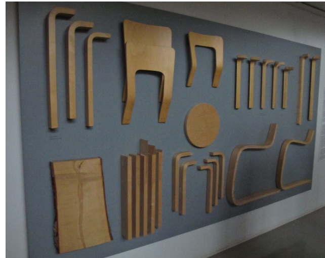
Alvar Aalto Museum: Various chair designs and modular wood parts used in chair construction
