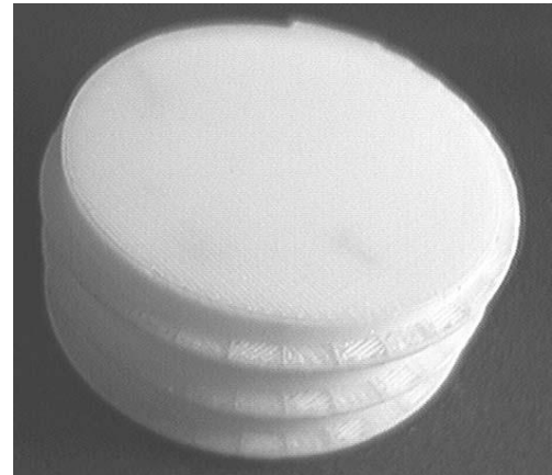
Figure 17. THE SCREW PART MANUFACTURED USING OUR ALGORITHM. USING THE QUICKSLICE SOFTWARE DIRECTLY, THE BUILD TOOK OVER TWICE AS LONG TO COMPLETE.
