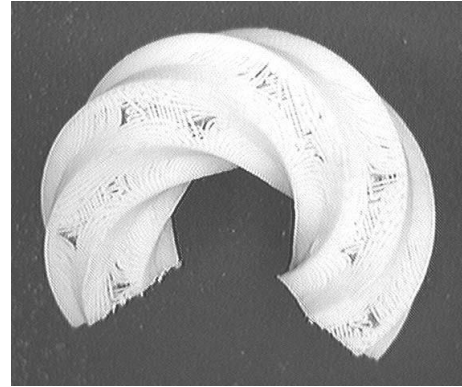
Figure 2. A PART BUILT WITH AN OVER-AGGRESSIVE MANUAL EXTENSION OF THE QUICKSLICE SOFTWARE’S FAST BUILD REGION. NOTE THE GAPS IN THE SURFACE ON THE NEAR-HORIZONTAL FACES.
