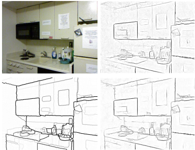
Fig. 2. Qualitative comparison of contours: Top row: color image, contours from [9], bottom row: contours from [18] and contours from our proposed contour detector.
