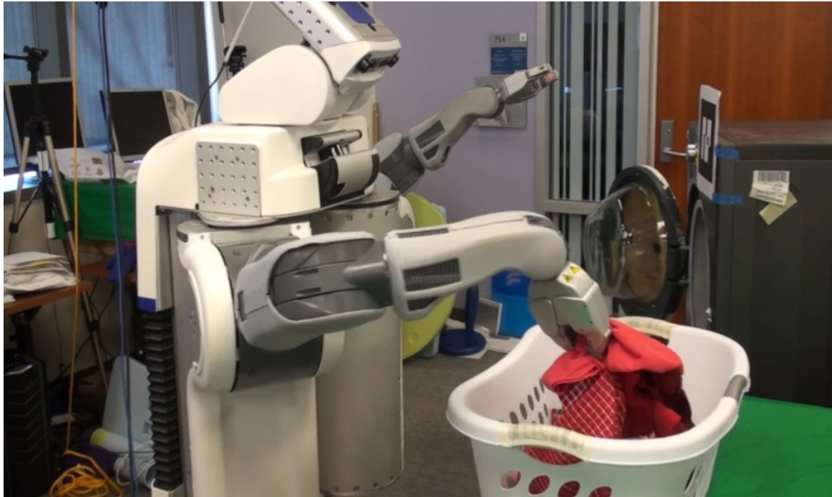
PR2: Two 8 DoF arms + 1 DoF height + 3 DoF base
