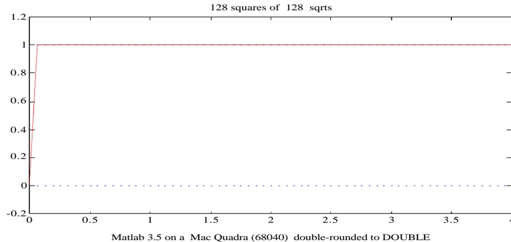
Without access to different roundings, how could someone tell that roundoff has spoiled the computation of  $H(X)$  ? Recomputation in higher precision might help, but a roughly correct graph would require at least about 40 sig. dec.
