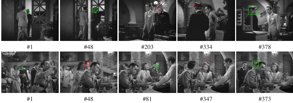
Figure 3. Tracking examples combining detection and correlation tracking. A detection step (when the track finds and matches a face detection close by) is shown in green, and a track step (using correlation) is shown in red. First row: #1, initial detection; #48, detection avoids drifting under poor image quality and background change; #203, the face, under a strange pose, is not detected, and the tracker switches to correlation tracking; #334, tracking continues when the head turns 180 degrees; #378, a detection corrects tracking and fixates it back on the person. Second row: a dynamic model helps tracking under occlusions. The track is lost after #48 and restarts at #81. After that, the track successfully goes through the shot, under severe occlusions such as in #347-#373.
