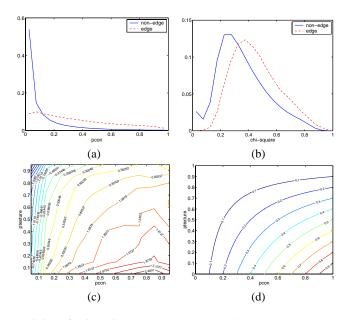
**Fig. 4.** Image statistics of orientation energy ( $p_{con,\theta}$ ) and textureness ( $p_{texture,\theta}$ ). (a) the marginal distributions of  $p_{con,\theta}$ , both the edge case and non-edge case. (b) the marginal distributions of the  $\chi^2$  distance used in Equation eqrefeq:ptexture to produce of  $p_{texture,\theta}$ . (c) the contour plot of the likelihood ratio  $\frac{P(\cdot|edge)}{P(\cdot|non-edge)}$ . (d) the contour plot of the multiplicative cue combination (Equation (6)).
