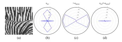
**Fig. 3.** Illustration of  $p_{texture,\theta}$ . (a) a patch from a zebra image; we consider the pixel at the center. (b) the distribution of raw  $p_{con,\theta}$  (not gated with  $p_{texture}$ ), maximal in the vertical direction. (c)  $1 - p_{texture,\theta}$ , maximal in the horizontal direction. (d) the product  $p_{b,\theta} = p_{con,\theta}(1 - p_{texture,\theta})$ , sharply peaked in the horizontal direction.
