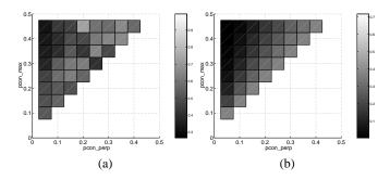
**Fig. 6.** The uncertainty of local orientation  $\sigma_{\theta}^2$  as a function of  $p_b^*$  and  $p_b^{\perp}$ . (a) the statistics from real images. (b) fitting the parametric model (Equation (8)).
