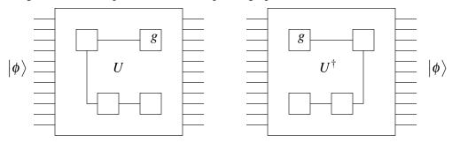
The circuits for U and  $U^{\dagger}$  are the same size and have mirror image gates. Examples:
